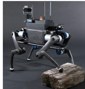
Examples of hybrid systems that can be controlled by MPC controllers: bipedal robots (left, Kouppas et al., Rob Auton Syst, 2021] and quadruped robots (right, ANYmal developed by ETH Zurich)
