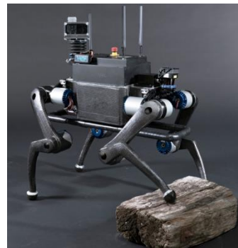
Figure 2 ANYmal developed by ETH Zurich
